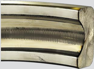
Bearing fluting, "washboard" pattern on bearing race
