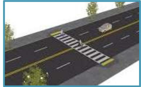
**Figure 17. Lane Reconfiguration Road Diet Example**
