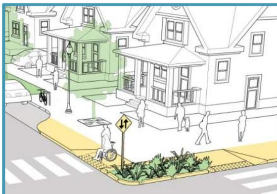
**Figure 19. Bulb Out Example**
