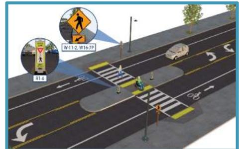
**Figure 18. Pedestrian Crossing Road Diet Example**
