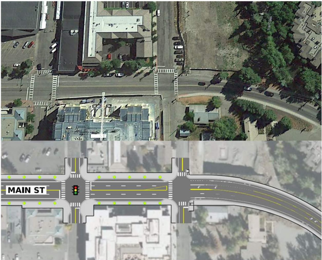
Figure 20. Existing Merge Between 1 st and River (Top) and Proposed Merge South of River (Bottom)
