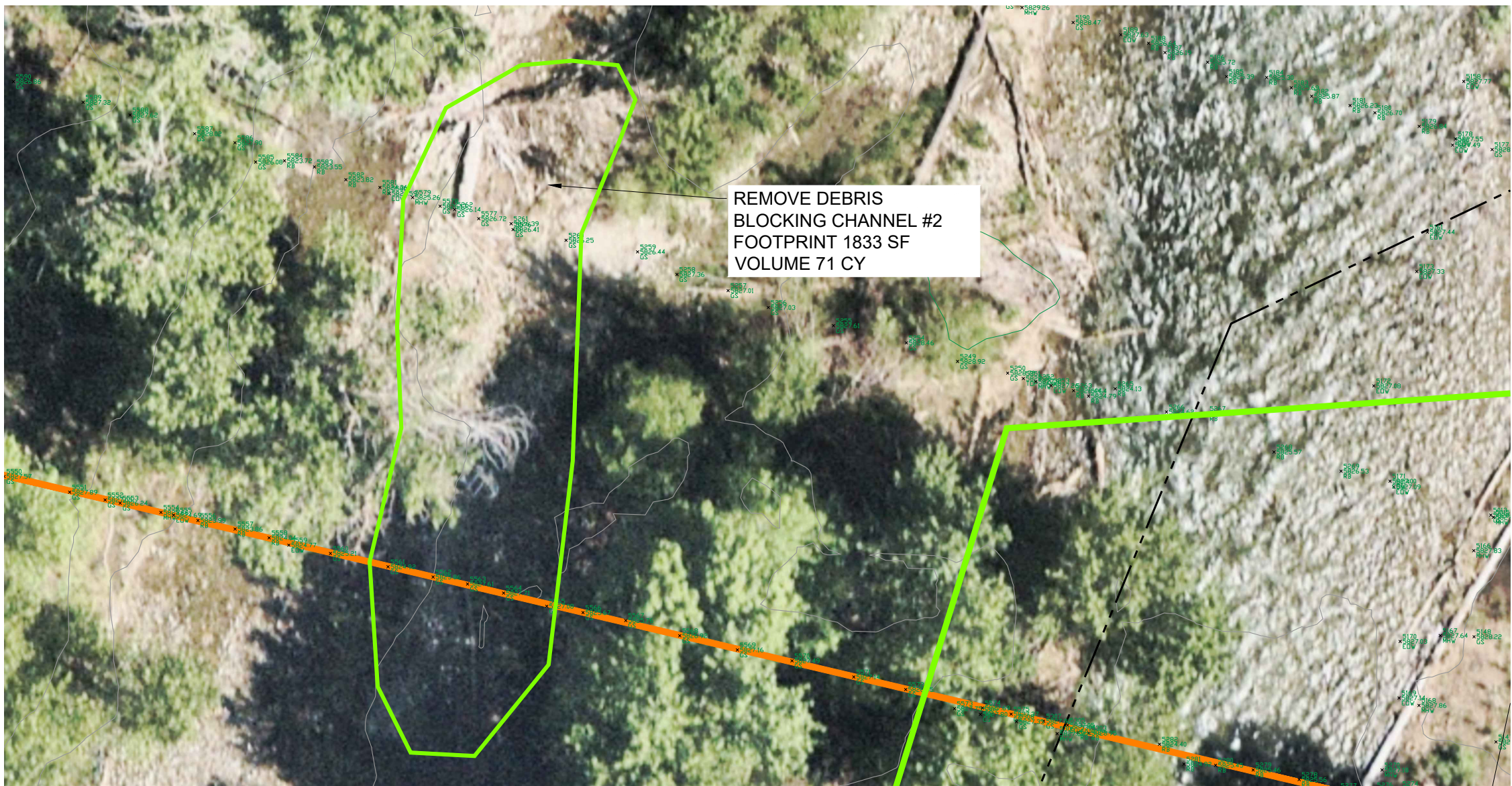
AREA 2: CHANNEL #2 BLOCKAGE SCALE: 1" = 10'
