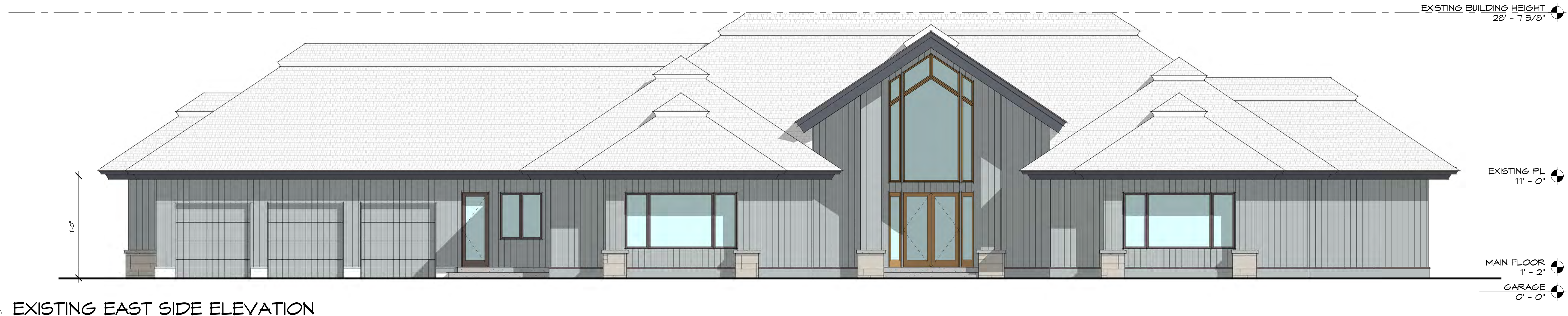
1 X2 EXISTING EAST SIDE ELEVATION 3/16" = 1'-0"
