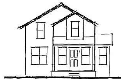
Residential façade with appropriate level of articulation
