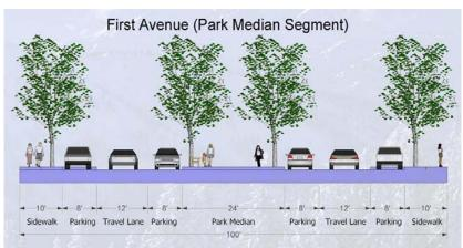
Figure 3.K: Park Median Segment/First Avenue cross-section, Four lanes of parallel parking will replace two lanes each of diagonal and parallel parking. The reduction in parking units will allow for a center median to enhance the neighborhood through provision of an attractive, informal open space.
