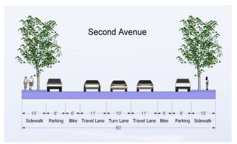
**Figure 3.M: Second Avenue Segment** cross-section, with three lanes allowing for a dedicated left-turn lane. It is possible to include some medians in the turn lane to enhance the gateway character of this important avenue.
