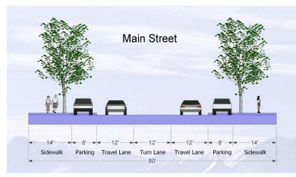
Figure 3.N: Main Street Segment cross-section, with three lanes allowing for a dedicated left-turn lane.
